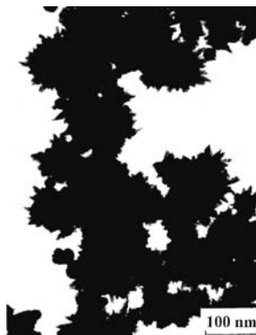
Figure 2. TEM image of the gladiate product obtained by hydrothermal approach.
