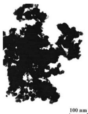
Figure 3. TEM image of the as-prepared Ru particles in open system.
